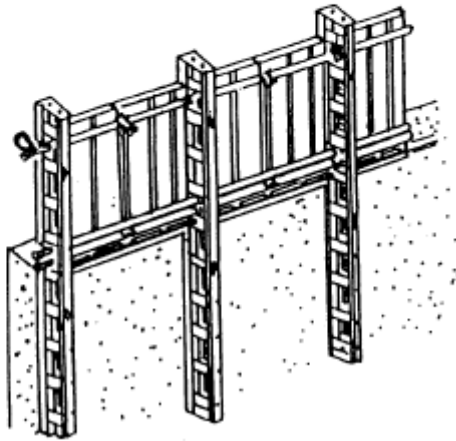
Fig. 5.1A : Single Sided Wall Form (Adjustable)
